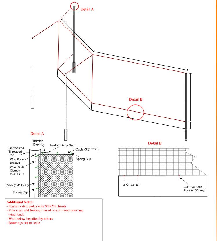
Tie Back Net Backstop System With Wall Below
