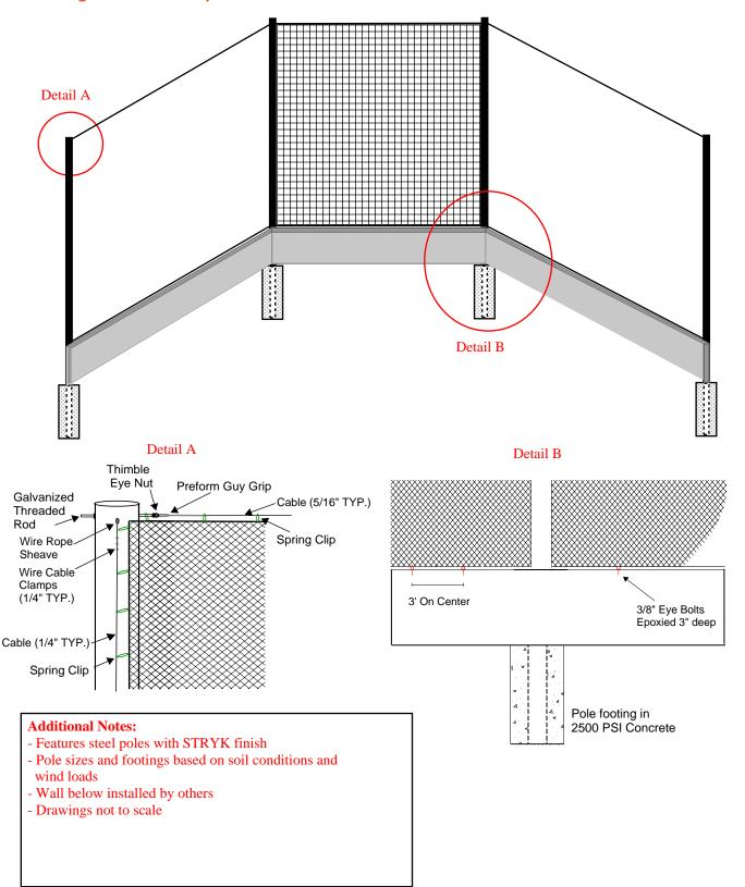
In-line Net Backstop System With Wall Below
