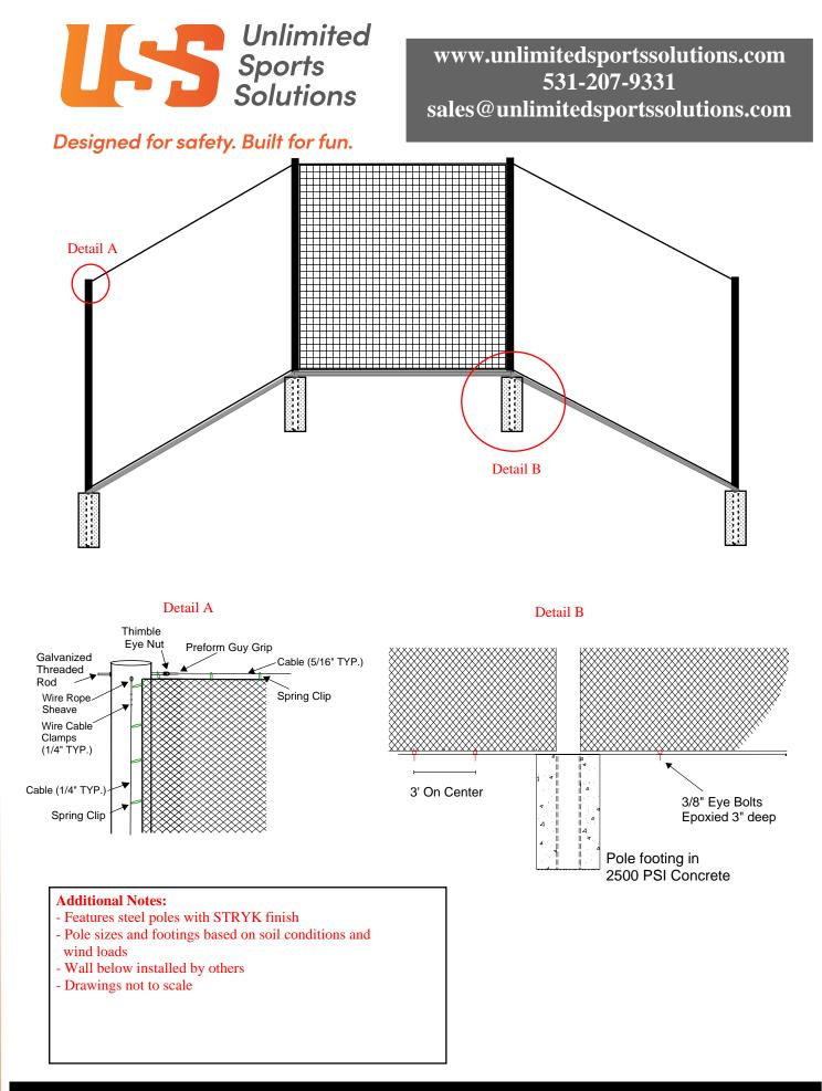
In-line Net Backstop System With Net to Mow Curb
