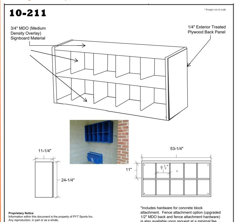
Painted With Two Coats Of Exterior Enamel Paint Mounting Styles Available For: Concrete Block, Wood Or Fence Dugouts No Assembly Required Each Order Includes One Can of "Touch Up" Paint For Post Installation
